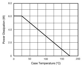
Fig. 1 - Power Derating Curve
