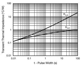
Fig. 5 - Typical Transient Thermal Impedance
