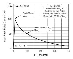
Fig. 3 - Pulse Waveform
