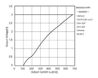
Figure 5. Output Voltage vs. Output Current (OCP Threshold)
