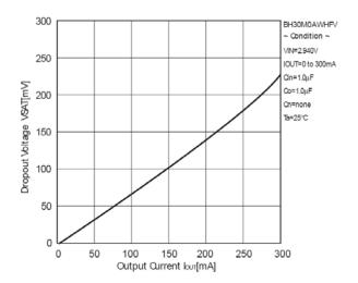
Figure 6. Dropout Voltage vs. Output Current
