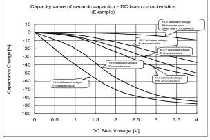
Figure 11. Capacity-bias characteristics
