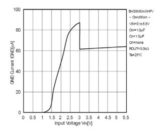
Figure 4. GND Current vs. Input Voltage
