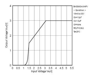
Figure 3. Output Voltage vs. Input Voltage
