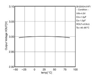
Figure 7. Output Voltage vs. Temperature
