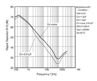
Figure 8. Ripple Rejection vs. Frequency
