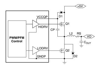
Figure 4. Charge Pump Configuration
