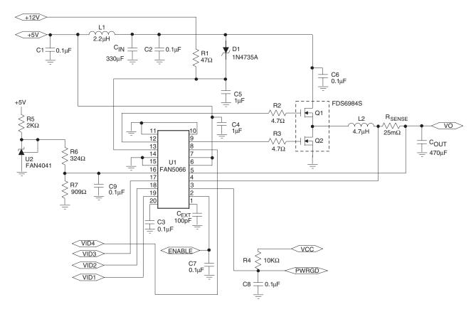
Figure 1. Application Circuit for 900mV @ 3A
