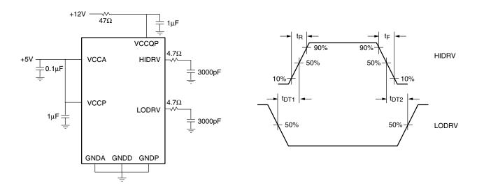
Figure 3. Output Drive Test Circuit and Timing Diagram
