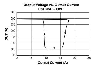
Figure 6. FAN5066 Short Circuit Characteristic
