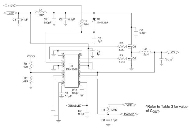
Figure 2. 12A Application Circuit for DDR VTT
