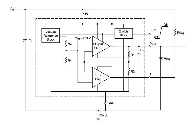
Figure 2. Typical Schematic, Fixed Output Version
