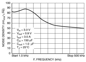
Figure 10. Noise Density vs. Frequency
