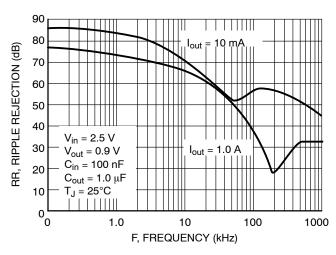
Figure 8. Ripple Rejection vs. Frequency
