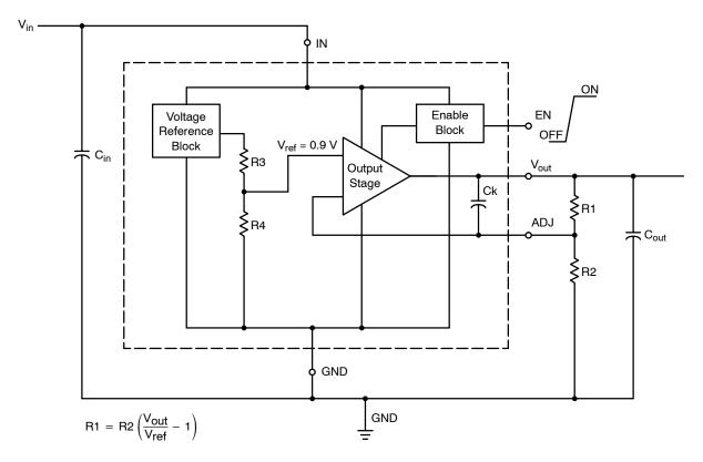
Figure 1. Typical Schematic, Adjustable Output Version
