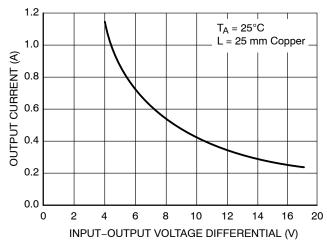
Figure 7. Output Current vs. Input-Output Voltage Differential
