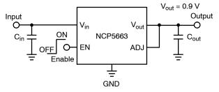
Figure 17. To achieve the minimum output voltage, ADJ to V<sub>out</sub> has to be connected together
