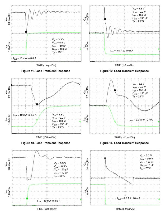
Figure 15. Load Transient Response
