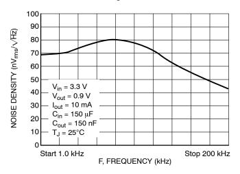
Figure 9. Noise Density vs. Frequency
