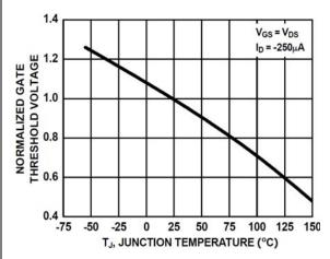
Figure 11. Normalized Gate Threshold Voltage vs
