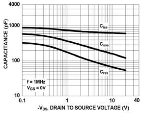
Figure 13. Capacitance vs Drain to Source Voltage
