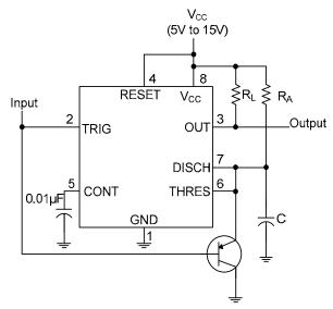
Fig. 7 Circuit for Missing Pulse Dectector
