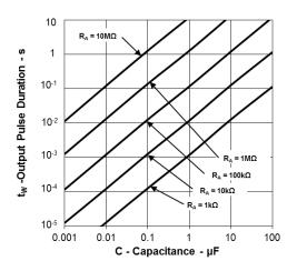
Fig. 3 Output Pulse Duration vs. Capacitance
