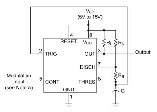
The modulating signal can be directly or capacitively coupled to CONT. For direct coupling, the effects of modulation source voltage and impedance on the bias of the timer should be considered.
