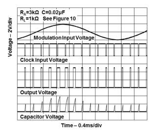
Fig 11. Pulse width modulation timing diagrams
