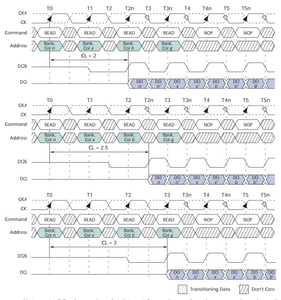
Notes: 1. DO n (or x or b or g) = data-out from column n (or column x or column b or column g).
