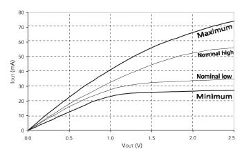
Figure 16: Reduced Drive Pull-Up Characteristics
