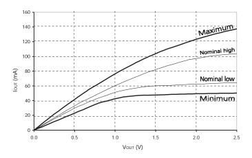
Figure 14: Full Drive Pull-Up Characteristics
