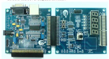
2. Connect your PC to the CY3280-22x45 Universal CapSense Controller board's ISSP connector (J3) using a PSoC MiniProg and an USB cable.
