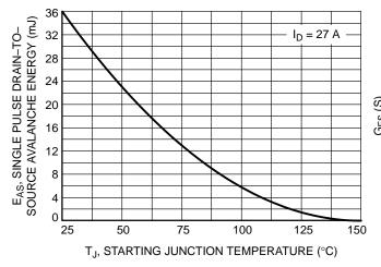
Figure 11. Maximum Avalanche Energy vs. Starting Junction Temperature
