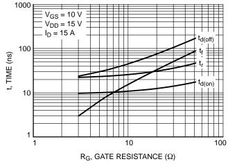
Figure 8. Resistive Switching Time Variation vs. Gate Resistance
