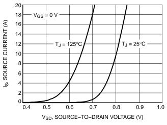
Figure 9. Diode Forward Voltage vs. Current
