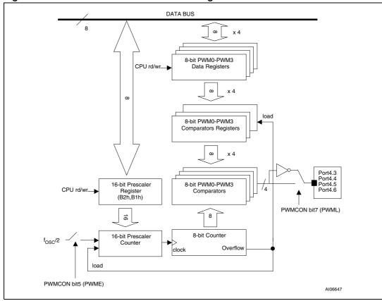
Figure 35. Four-channel 8-bit PWM block diagram
