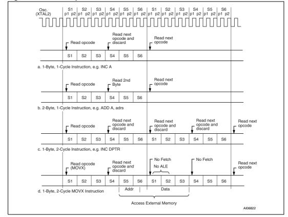
Figure 13. State sequence in UPSD321xx devices
