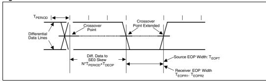
Figure 43. Differential to EOP transition skew and EOP width
