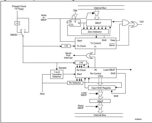
Figure 30. Serial port Mode 2 block diagram
