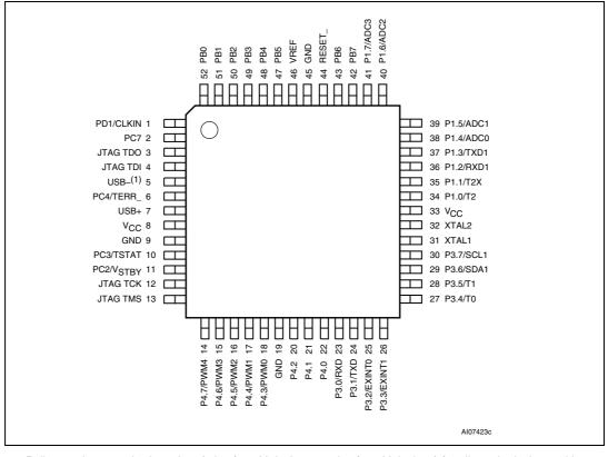
Figure 2. TQFP52 connections
