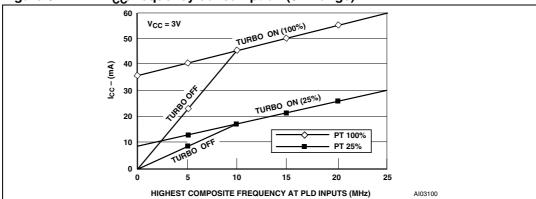
Figure 67. PLD I<sub>CC</sub>/frequency consumption (3 V range)
