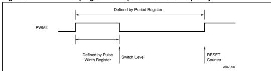
Figure 37. PWM 4 with programmable pulse width and frequency
