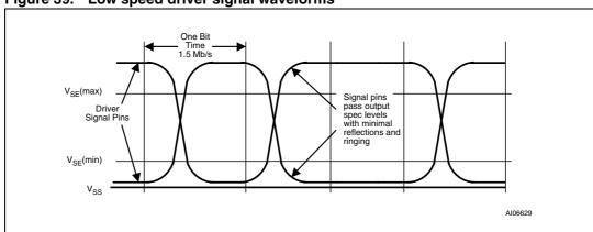
Figure 39. Low speed driver signal waveforms
