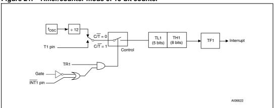
Figure 21. Timer/counter mode 0: 13-bit counter
