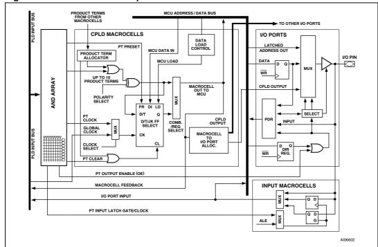
Figure 54. Macrocell and I/O ports
