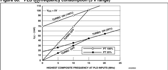
Figure 66. PLD I<sub>CC</sub>/frequency consumption (5 V range)
