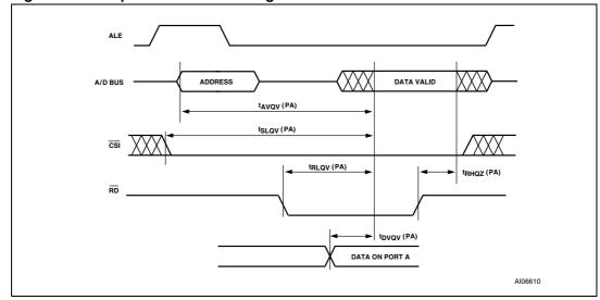
Figure 77. Peripheral I/O Read timing
