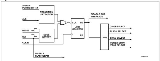
The PSD module has a Turbo Bit in PMMR0. This bit can be set to turn the Turbo mode off (the default is with Turbo mode turned on). While Turbo mode is off, the PLDs can achieve standby current when no PLD inputs are changing (zero DC current). Even when inputs do change, significant power can be saved at lower frequencies (AC current), compared to when Turbo mode is on. When the Turbo mode is on, there is a significant DC current component and the AC component is higher.
