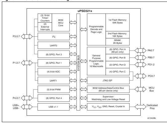
Figure 1. UPSD321xx block diagram
