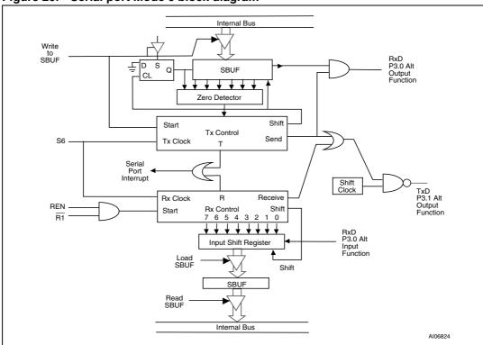
Figure 26. Serial port Mode 0 block diagram
