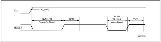
Table 103. Status during Power-on RESET, Warm RESET and Power-down mode
