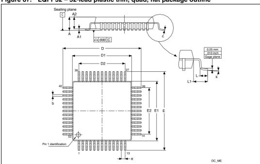
Figure 87. LQFP52 – 52-lead plastic thin, quad, flat package outline
