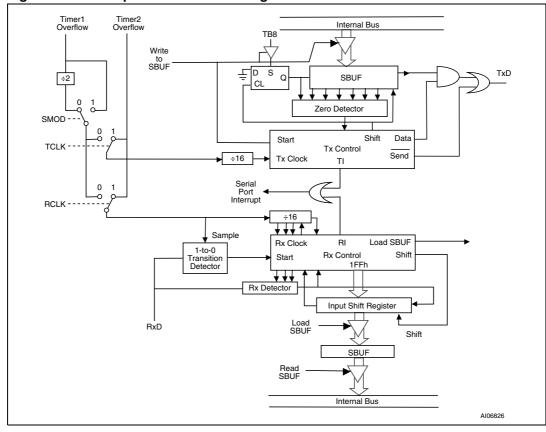
Figure 28. Serial port Mode 1 block diagram
