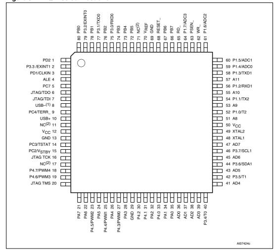
Figure 3. TQFP80 connections
