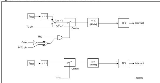
Figure 23. Timer/counter mode 3: two 8-bit counters
