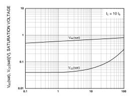
Figure 3. Base-Emitter Saturation Voltage Collector-Emitter Saturation Voltage
