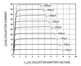
Figure 1. Static Characteristic
