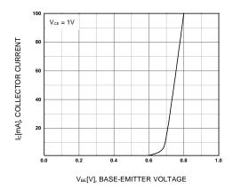
Figure 4. Base-Emitter On Voltage
