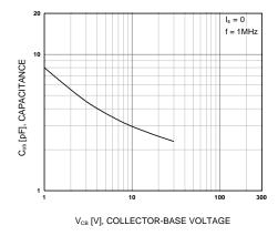
Figure 5. Collector Output Capacitance
