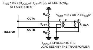
FIGURE 14. ALTERNATIVE OUTPUT LOADING
