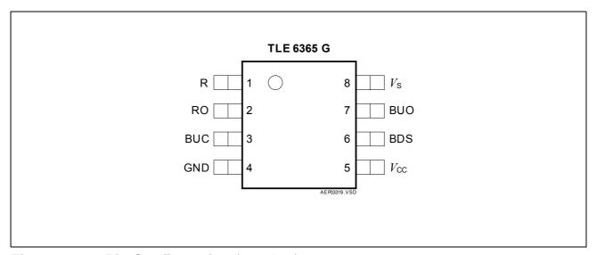
Figure 1 Pin Configuration (top view)
