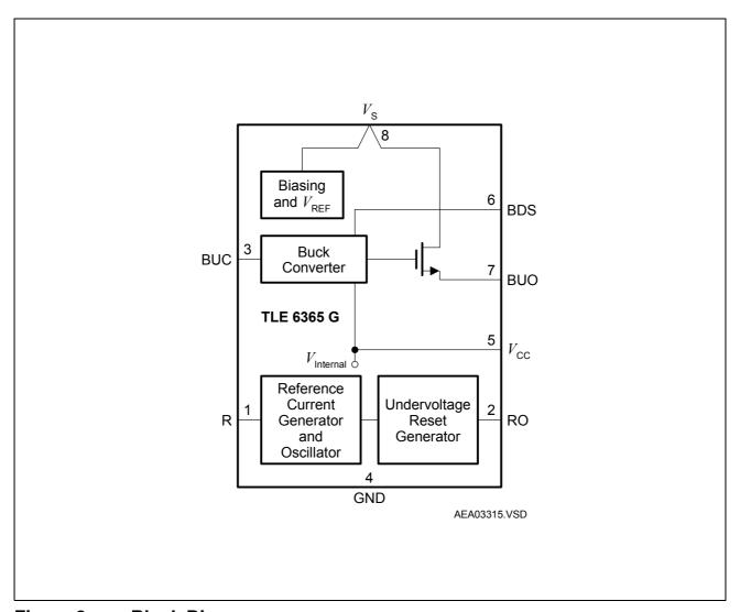
Figure 2 Block Diagram
