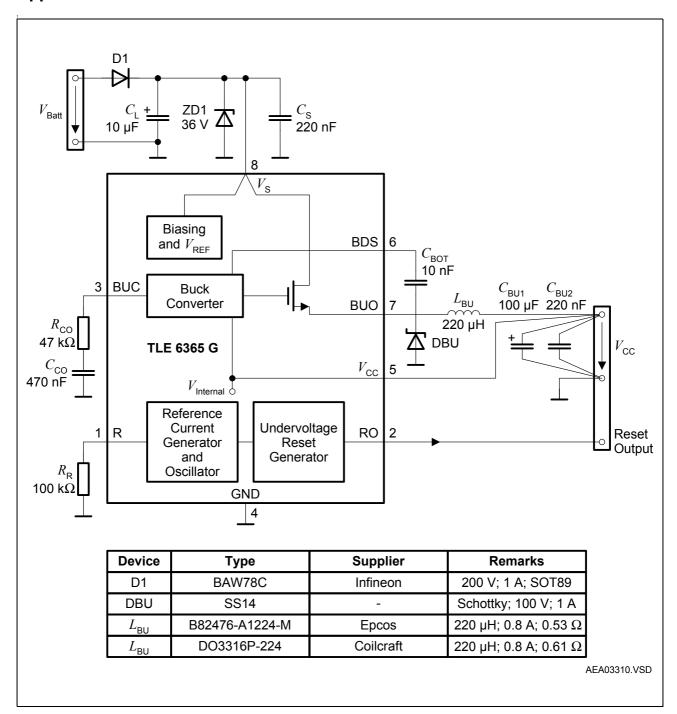
Figure 6 Application Circuit
