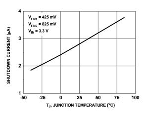
Figure 9. Shutdown Current vs Temperature
