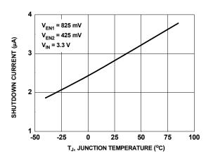
Figure 10. Shutdown Current vs Temperature
