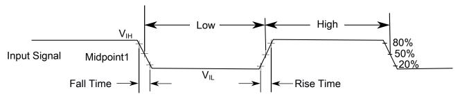
The midpoint is  $V_{IL}$  + ( $V_{IH}$  -  $V_{IL}$ ) / 2
