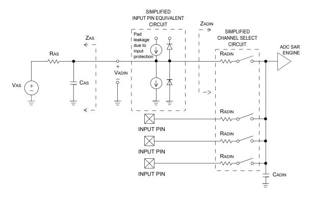
Figure 24. ADC input impedance equivalency diagram
