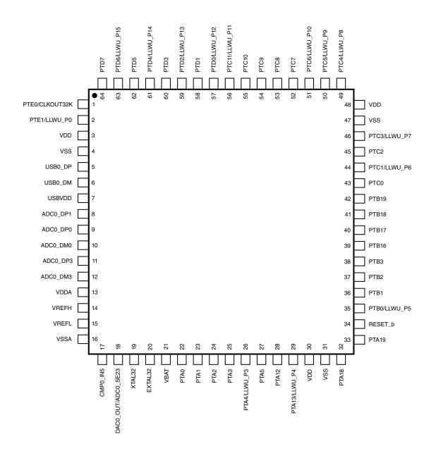
Figure 7. 64 LQFP Pinout Diagram
