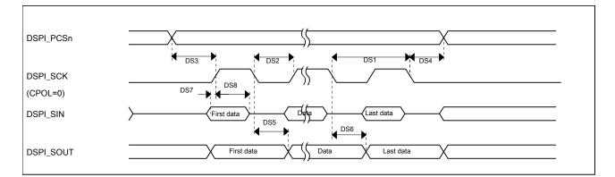
Figure 31. DSPI classic SPI timing — master mode
