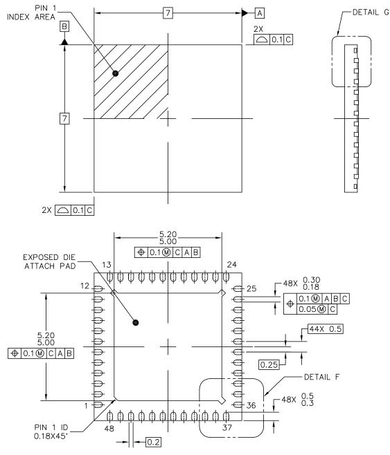
Figure 13. 48-pin QFN package dimension 1
