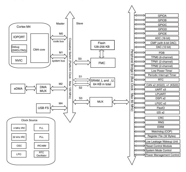
Figure 2. System diagram
