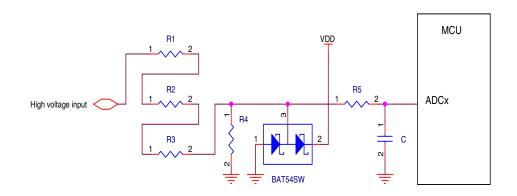
Figure 42. High voltage measurement with an ADC input
