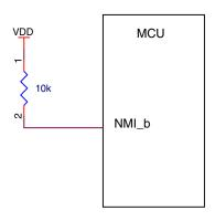
Figure 45. NMI pin biasing
