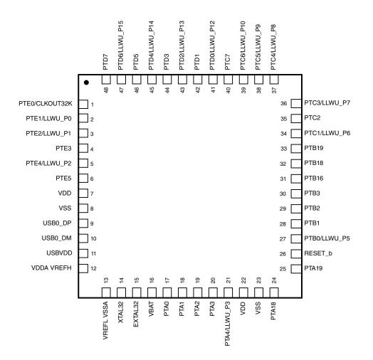
Figure 8. 48 QFN Pinout Diagram
