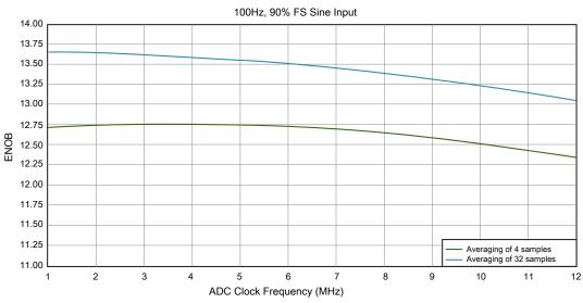
Typical ADC 16-bit Single-Ended ENOB vs ADC Clock
