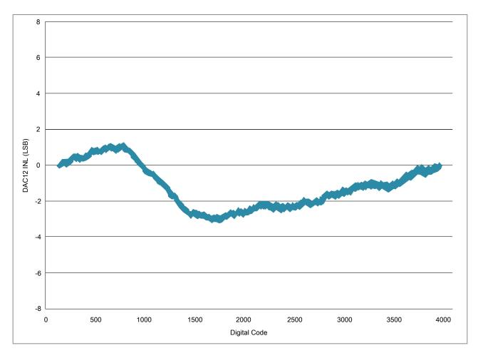
Figure 29. Typical INL error vs. digital code
