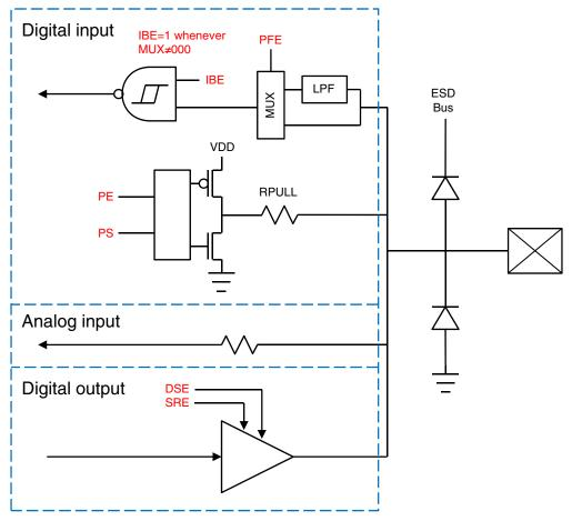
Figure 4. I/O simplified block diagram
