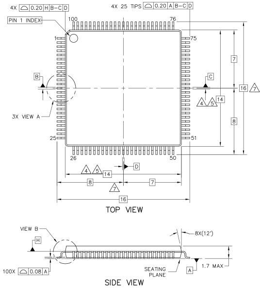
Figure 9. 100-pin LQFP package dimensions 1
