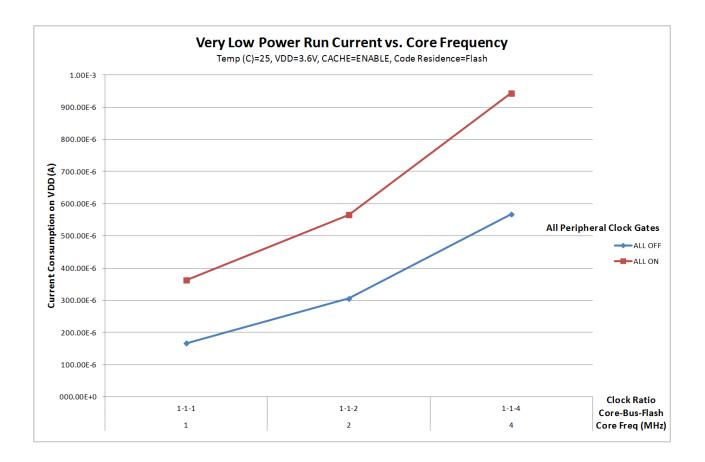
Figure 17. VLPR mode supply current vs. core frequency
