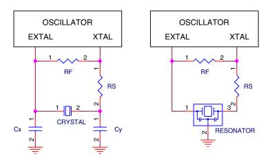
Figure 50. Crystal connection – Diagram 4
