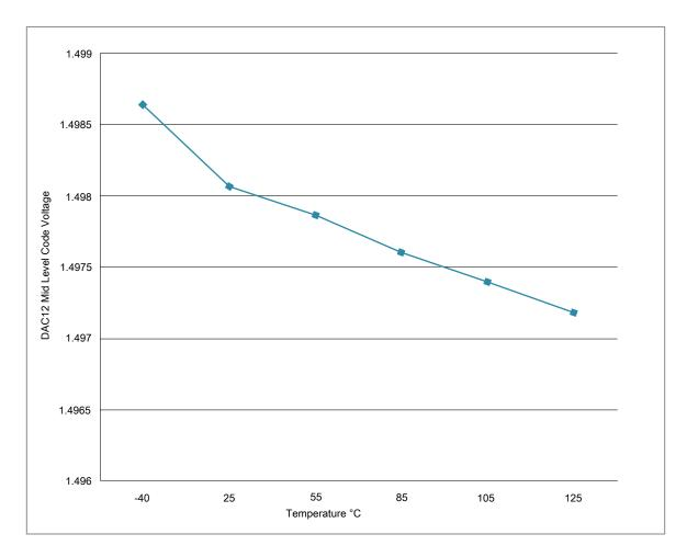
Figure 30. Offset at half scale vs. temperature
