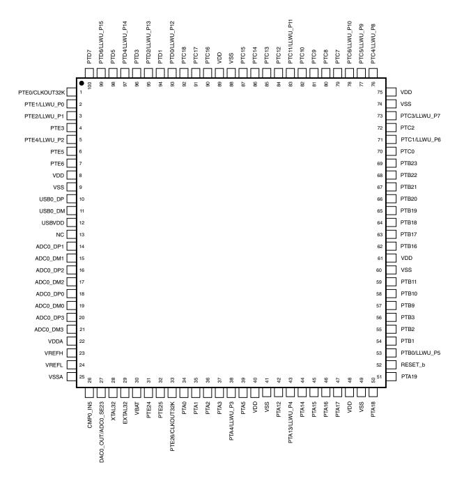
Figure 6. 100 LQFP Pinout Diagram
