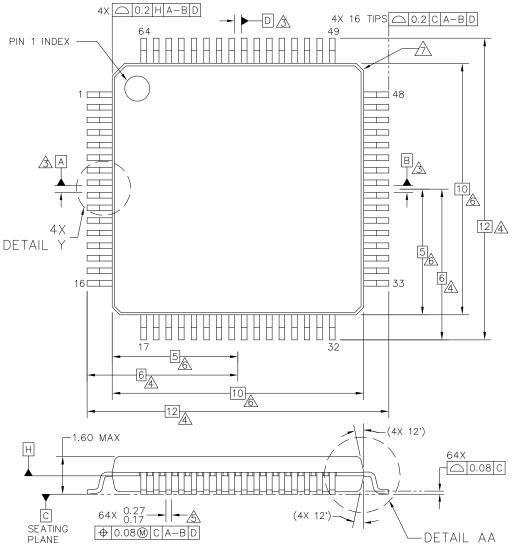
Figure 11. 64-pin LQFP package dimensions 1
