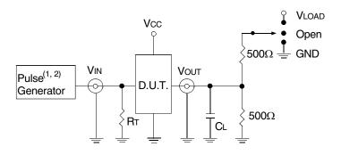
**Test Circuits for All Outputs**
