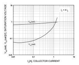
Figure 3. Base-Emitter Saturation Voltage Collector-Emitter Saturation Voltage
