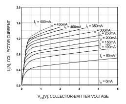
Figure 1. Static Characteristic
