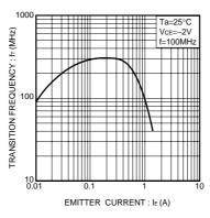
Fig.5 Gain bandwidth product vs. emitter current
