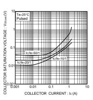
Fig.3 Collector-emitter saturation voltage vs. collector current
