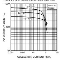
Fig.1 DC current gain vs. collector current
