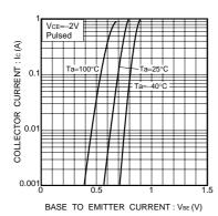
Fig.4 Grounded emitter propagation characteristics
