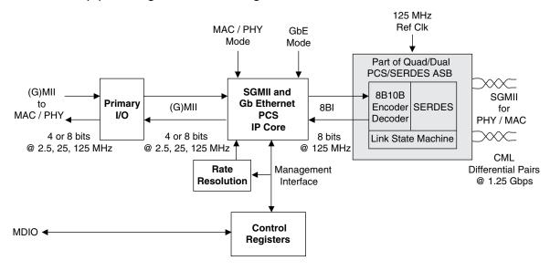
Figure 2-3 shows typical clock network connections between the IP core, the SERDES, and a MAC.
