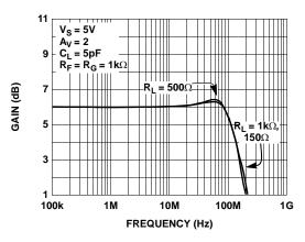
FIGURE 6. SMALL SIGNAL FREQUENCY RESPONSE vs VARIOUS  $R_{\text{LOAD}}$
