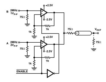
FIGURE 32. TWO TO ONE MULTIPLEXER
