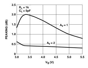
FIGURE 14. SMALL SIGNAL PEAKING vs SUPPLY VOLTAGE
