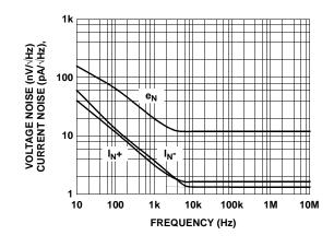
FIGURE 20. VOLTAGE AND CURRENT NOISE vs FREQUENCY
