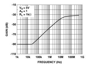
FIGURE 10. DISABLED OUTPUT ISOLATION FREQUENCY RESPONSE
