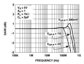
FIGURE 1. FREQUENCY RESPONSE FOR VARIOUS OUTPUT VOLTAGE LEVELS
