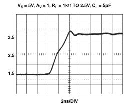
FIGURE 21. LARGE SIGNAL TRANSIENT RESPONSE - RISING
