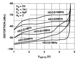
FIGURE 17. HARMONIC DISTORTION vs OUTPUT VOLTAGE
