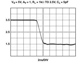
FIGURE 22. LARGE SIGNAL TRANSIENT RESPONSE - FALLING
