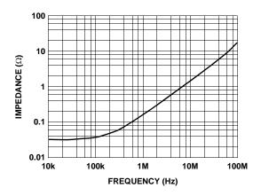
FIGURE 13. OUPUT IMPEDANCE vs FREQUENCY
