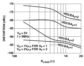
FIGURE 18. HARMONIC DISTORTION vs LOAD RESISTANCE
