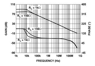
FIGURE 9. OPEN LOOP GAIN AND PHASE vs FREQUENCY
