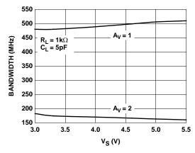
FIGURE 12. SMALL SIGNAL BANDWIDTH vs SUPPLY VOLTAGE
