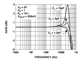
FIGURE 7. SMALL SIGNAL FREQUENCY RESPONSE vs  $C_L$
