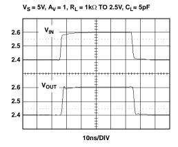
FIGURE 23. SMALL SIGNAL TRANSIENT REPONSE
