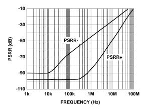
FIGURE 11. POWER SUPPLY REJECTION RATIO vs FREQUENCY
