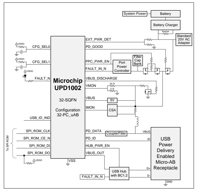
FIGURE 2-5: CONFIGURATION 32-PC\_UAB SYSTEM-LEVEL DIAGRAM
