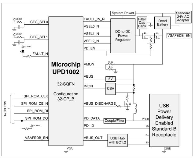
FIGURE 2-3: CONFIGURATION 32-CP\_B SYSTEM-LEVEL DIAGRAM
