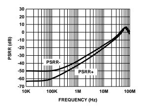
FIGURE 15. POWER SUPPLY REJECTION vs FREQUENCY
