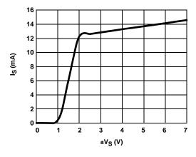
FIGURE 23. SUPPLY CURRENT vs SUPPLY VOLTAGE
