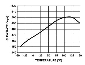
FIGURE 22. SLEW RATE vs TEMPERATURE
