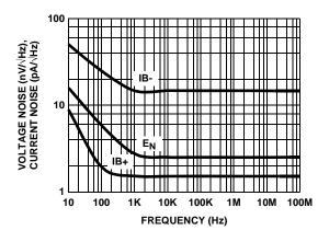
FIGURE 14. VOLTAGE AND CURRENT NOISE vs FREQUENCY
