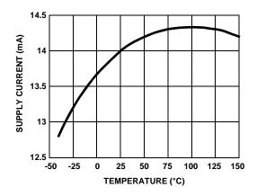
FIGURE 19. SUPPLY CURRENT vs TEMPERATURE
