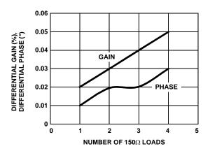
FIGURE 18. DIFFERENTIAL GAIN & PHASE
