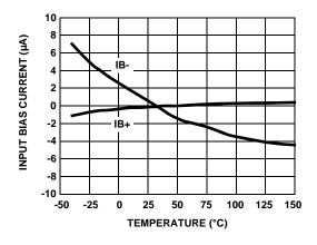
FIGURE 20. INPUT BIAS CURRENT vs TEMPERATURE
