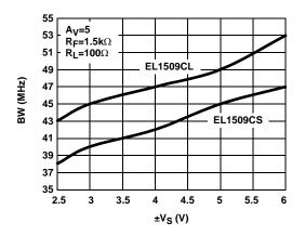
FIGURE 7. DIFFERENTIAL BANDWIDTH vs SUPPLY VOLTAGE
