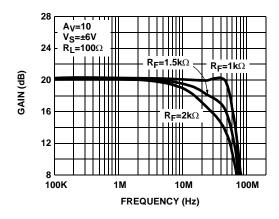
FIGURE 2. DIFFERENTIAL FREQUENCY RESPONSE vs R<sub>F</sub> (EL1509CL)
