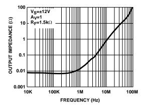
FIGURE 16. OUTPUT IMPEDANCE vs FREQUENCY
