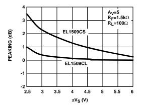
FIGURE 9. DIFFERENTIAL PEAKING vs SUPPLY VOLTAGE
