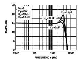
FIGURE 5. DIFFERENTIAL FREQUENCY RESPONSE vs C<sub>L</sub> (EL1509CS)
