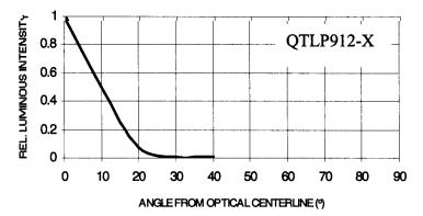
Fig 5. Relative Intensity vs. Angular Displacement
