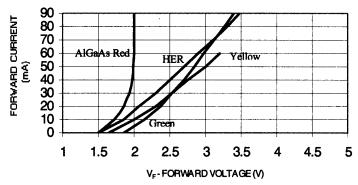
Fig 1. Forward Current vs. Forward Voltage
