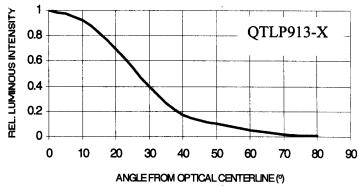
Fig 4. Relative Intensity vs. Angular Displacement
