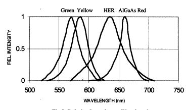
Fig 3. Relative Intensity vs. Wavelength
