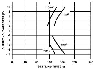
FIGURE 9. SETTLING TIME FOR VARIOUS OUTPUT STEP VOLTAGES
