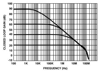
FIGURE 5. CLOSED LOOP FREQUENCY RESPONSE
