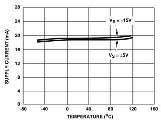
FIGURE 10. POWER SUPPLY CURRENT vs TEMPERATURE
