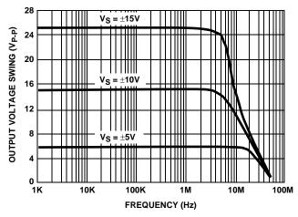
FIGURE 6. OUTPUT VOLTAGE SWING vs FREQUENCY
