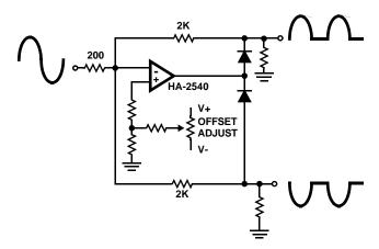
NOTE: With one HA-2540 and two low capacitance switching diodes, signals exceeding 10MHz can be separated. This circuit is most useful for full wave rectification, AM detectors or sync generation.
