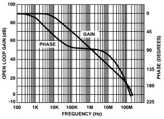
FIGURE 16. OPEN LOOP GAIN/PHASE vs FREQUENCY
