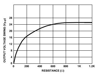
FIGURE 7. OUTPUT VOLTAGE SWING vs LOAD RESISTANCE
