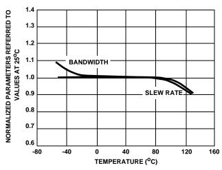
FIGURE 8. NORMALIZED AC PARAMETERS vs TEMPERATURE
