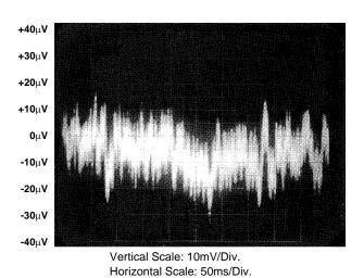
FIGURE 13. BROADBAND NOISE (0.1Hz TO 1MHz)
