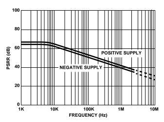
FIGURE 15. POWER SUPPLY REJECTION RATIO vs FREQUENCY
