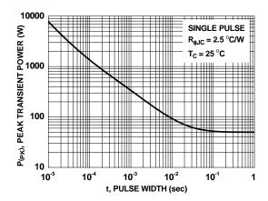
Figure 12. Single Pulse Maximum Power Dissipation
