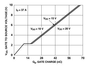
Figure 7. Gate Charge Characteristics
