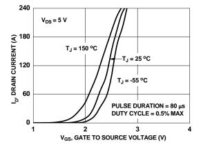
Figure 5. Transfer Characteristics
