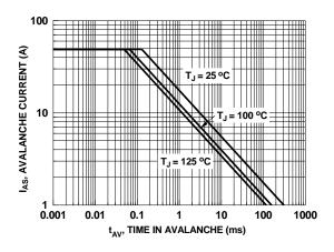
Figure 9. Unclamped Inductive Switching Capability
