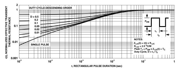
Figure 13. Junction to Case Transient Thermal Response Curve
